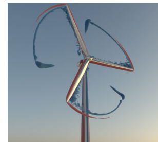
Nalu-Wind blade-resolved large-eddy simulation (LES) of the NREL 5-MW turbine
