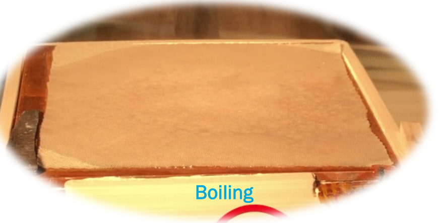
Fabric drying test in vacuum chamber
