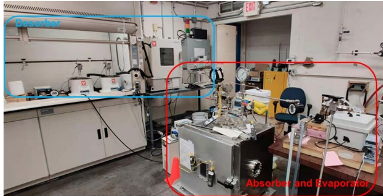
Photo of the developed prototype absorption chiller which utilizes the microemulsion-water as the working pair.
