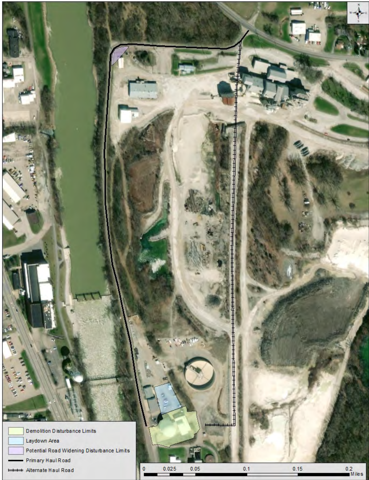
Figure 4. Limits of Disturbance for the Proposed Demolition of the Piqua Decommissioned Reactor Site
