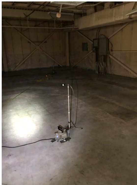
Photo 35. Air Clearance Testing
