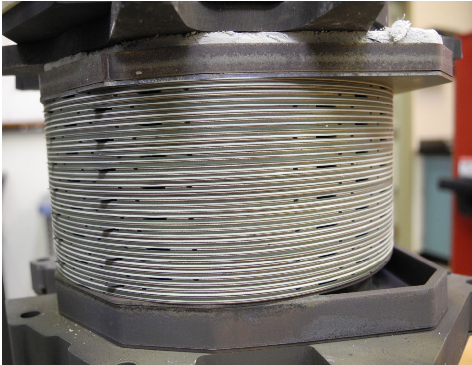
35-cell PCEC Stack – Core (Left) and Stack in Test Stand (Right)
