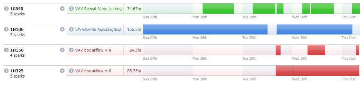
Figure 3. Zone-level fault detection and diagnostics
