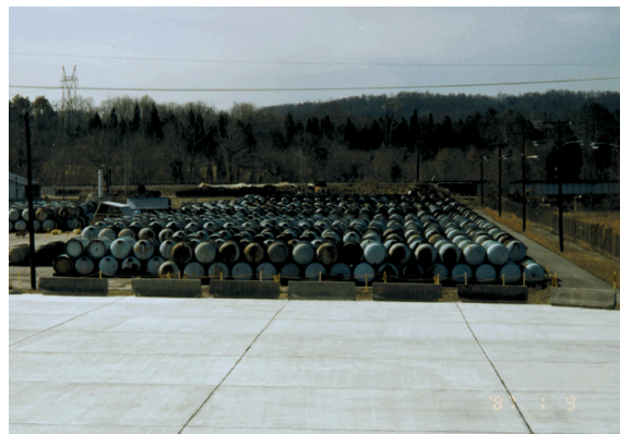
Depleted UF_6 is stored in cylinder yards like this one at Portsmouth.
