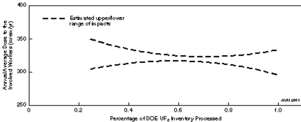
FIGURE K.62 Estimated Annual Average Individual Dose to Involved Workers from the Disposal of Grouted UO 2 (The ranges reflect differences in disposal technologies, i.e., shallow earthen structures, vaults, and mine.)
