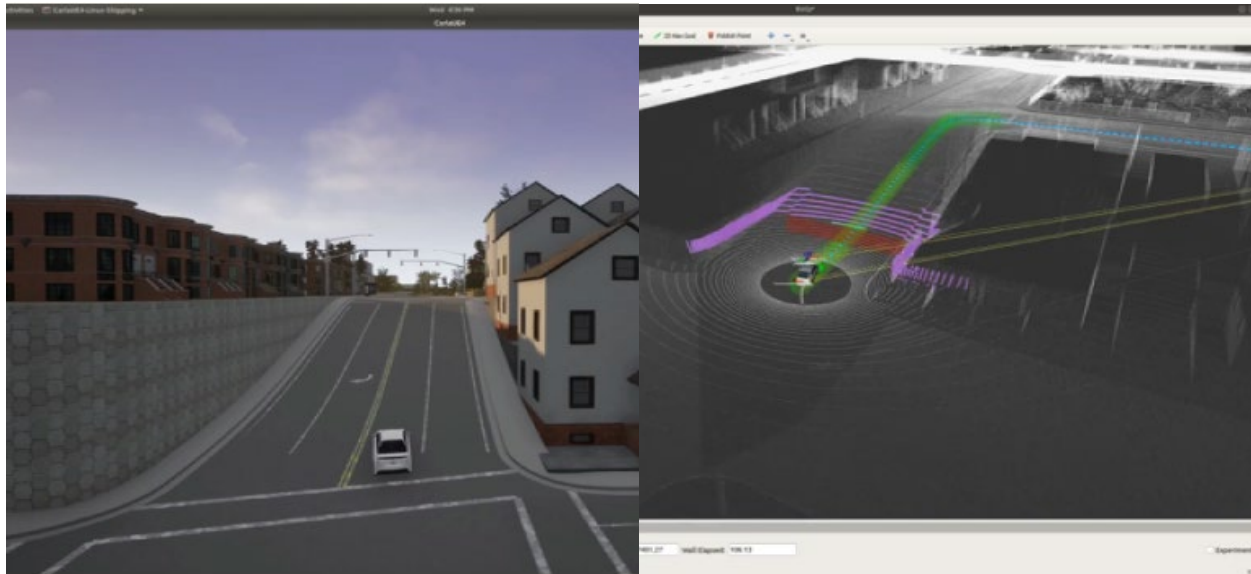
Figure I.3.3.4 Left: The CARLA Server with an Ego Vehicle Making a Right Turn. Right: The Autaware Rviz Configuration Displays All the Relevant Sensor Data to Localize the Ego Vehicle and Follow the Green Waypoints
