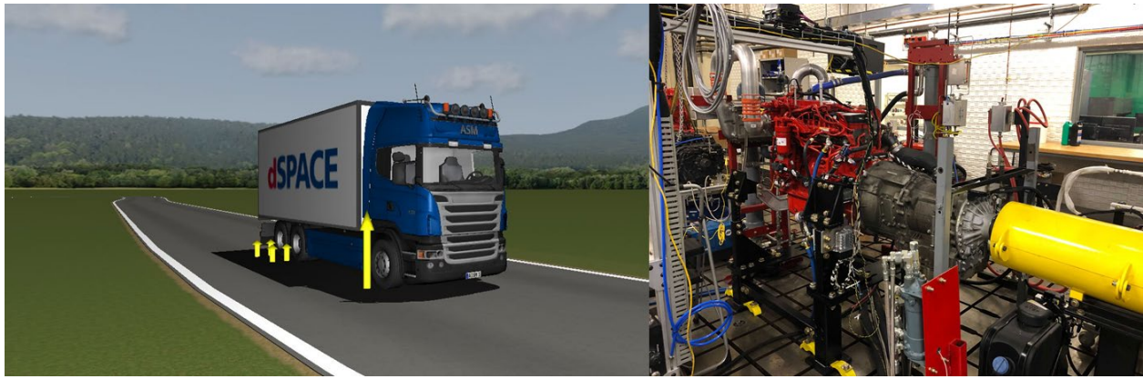
Figure I.3.3.1 Dspace ASM Virtual Vehicle-In-The-Loop (Left) Fully Integrated and Navigating a Handling Course Using Feedback from the Powertrain Under Test (Right)
