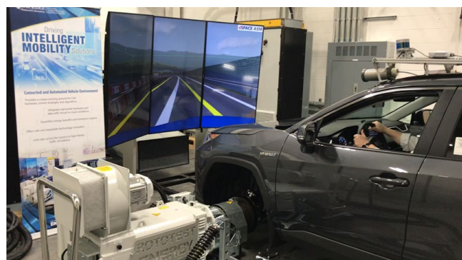
Figure 6 ORNL CAVE Lab with Vehicle-in-the-Loop Functionality
