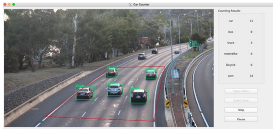
Figure I.2.4.9 Vehicle Detection/Counting Within a Predefined Area of Interest (Red Polygon)
