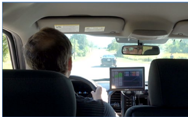
Figure I.3.2.4 Improved Data Acquisition and Control System with Heads-Up Control Touch Panel
