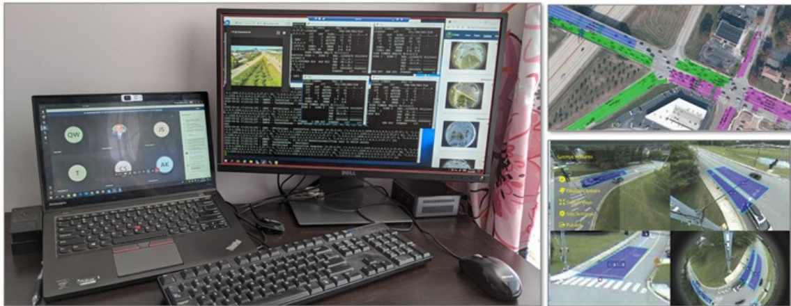
Figure I.2.5.4 Remote Setup of Control Experiment: VPN Tunnel into City of Chattanooga from Remote Desktop Interfaces to Run Control Algorithms in the Cloud and Obtain New Values to Send to On-Street Controllers
