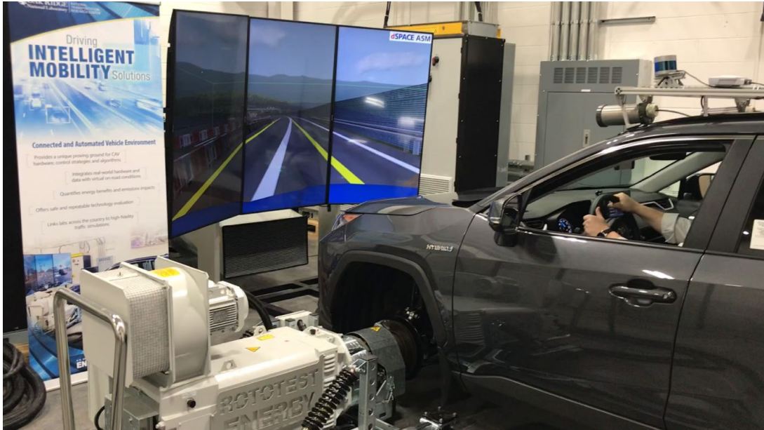
Figure I.3.3.2 CAVE Lab Setup with Full Vehicle-In-The-Loop (VIL) Functionality, Including Steering, Integrated with Virtual Vehicle Environment
