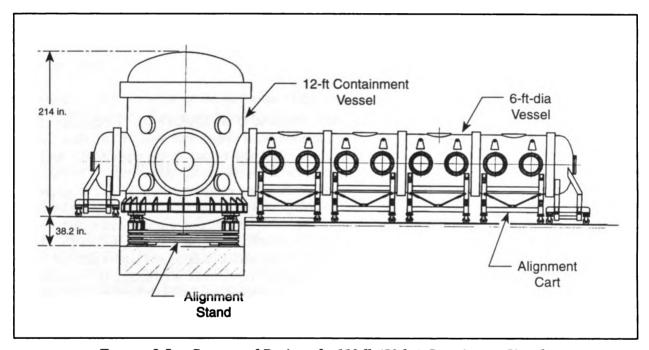
FIGURE 3-5.—Conceptual Design of a 110-lb (50-kg) Containment Vessel.
