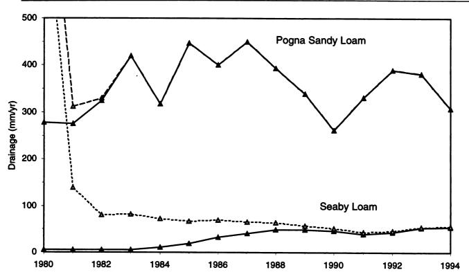
FIGURE E1-7.—Simulation Results Showing the Impact of Initial Conditions on Annual Drainage from the Pogna Sandy Loam and Seaby Loam Soil Profiles.
