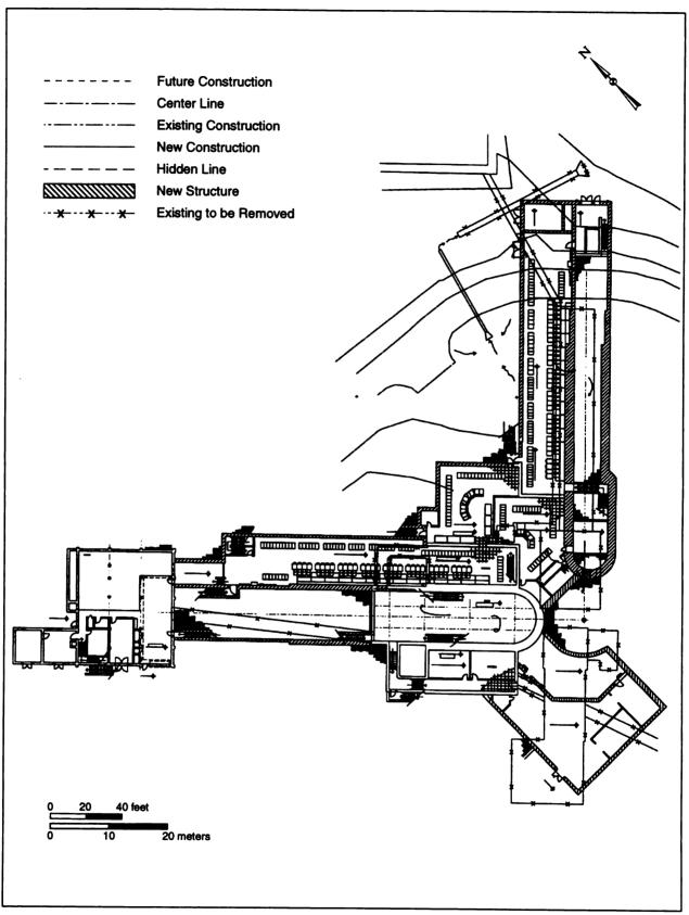
FIGURE 3-4.—Conceptual Design of the PHERMEX Upgrade Facility.
