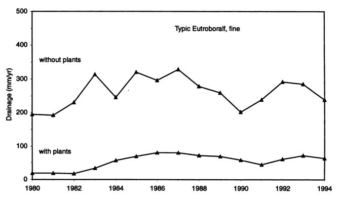
FIGURE E1-3.—Simulation Results Showing Annual Drainage from the Typic Eutroboralf Soil Profile.
