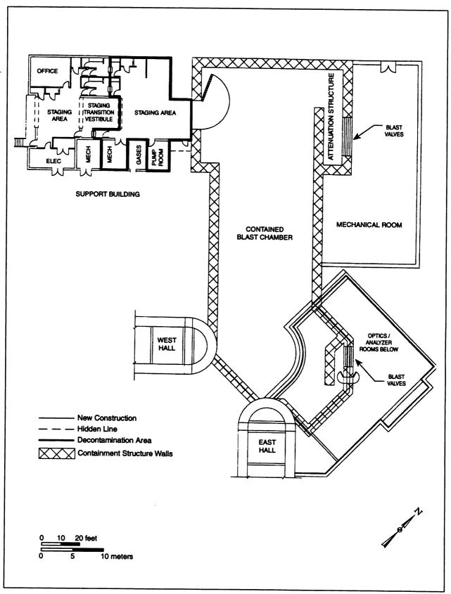
FIGURE 3-6.—Conceptual Design of the Containment Building.
