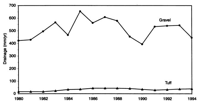
FIGURE E1-1.—Simulation Results Showing Annual Drainage from the Tuff and Gravel Soil Profiles.
