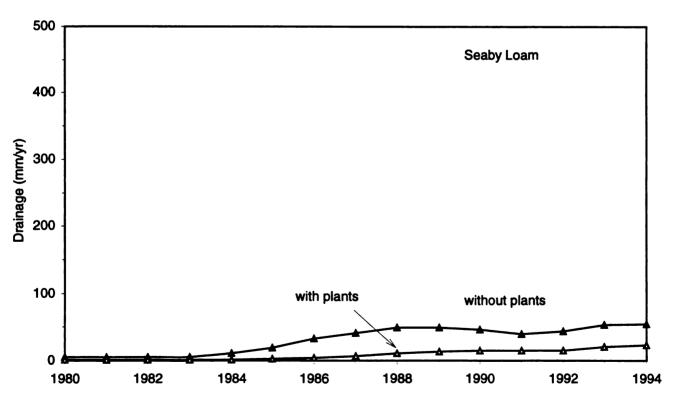
FIGURE E1-4.—Simulation Results Showing Annual Drainage from the Seaby Loam Soil Profile.
