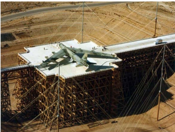
Air Force EMP testing a B-52 bomber to ensure it is EMP hardened and will continue to operate in a nuclear environment.
