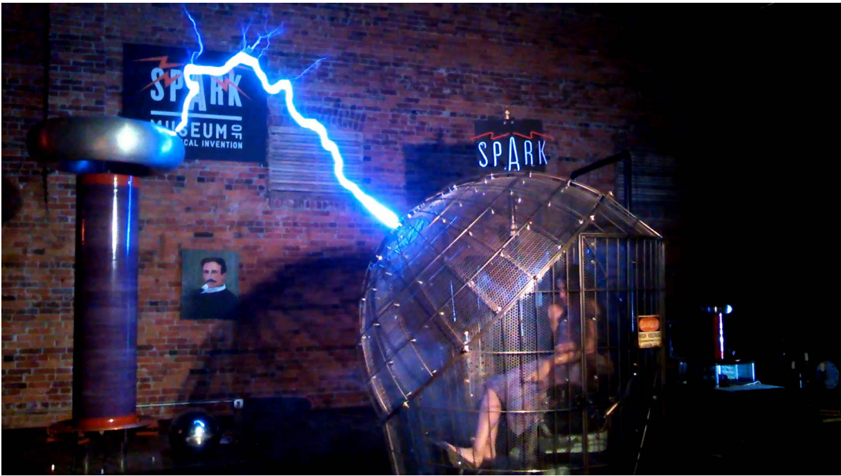
Faraday cages protect people or objects inside of them from electrical impacts. Similar cages can be used to protect transformers and communications centers or SCADAs. There are also other ways to protect indoor equipment that DARPA contractor Conductive Composites in Heber City, UT among others, has perfected.
