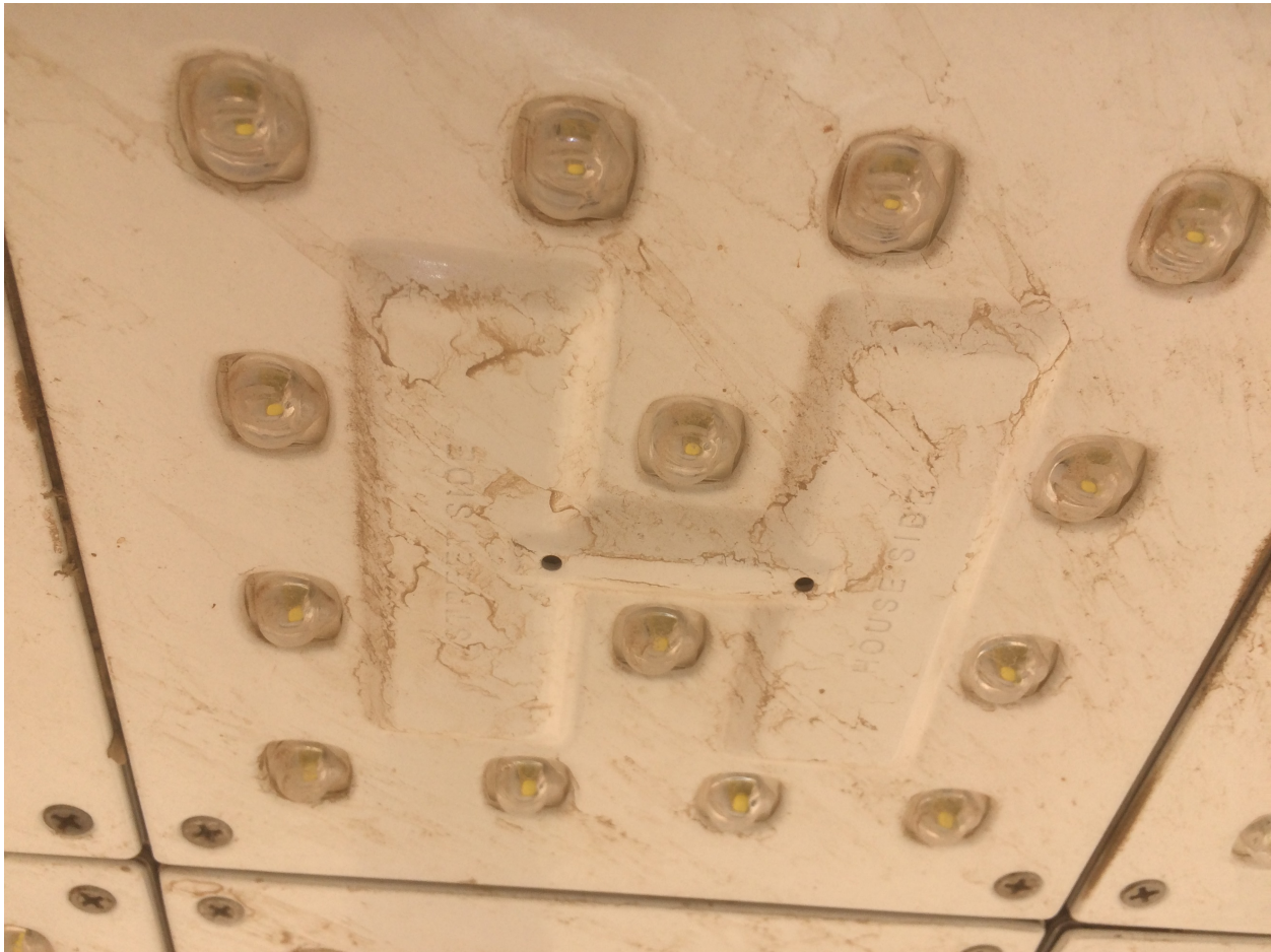
Figure 1. LED array with accumulated dirt from the project site in Yuma, AZ.
