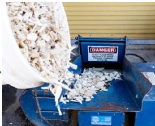
2-stage size reduction: chip and mill
