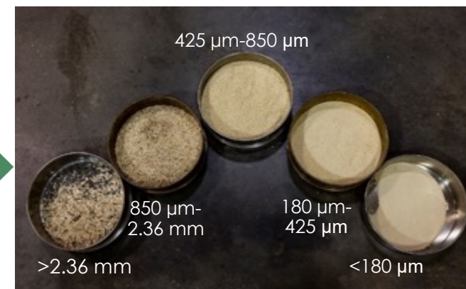
Particle size separation by vibratory shaker
