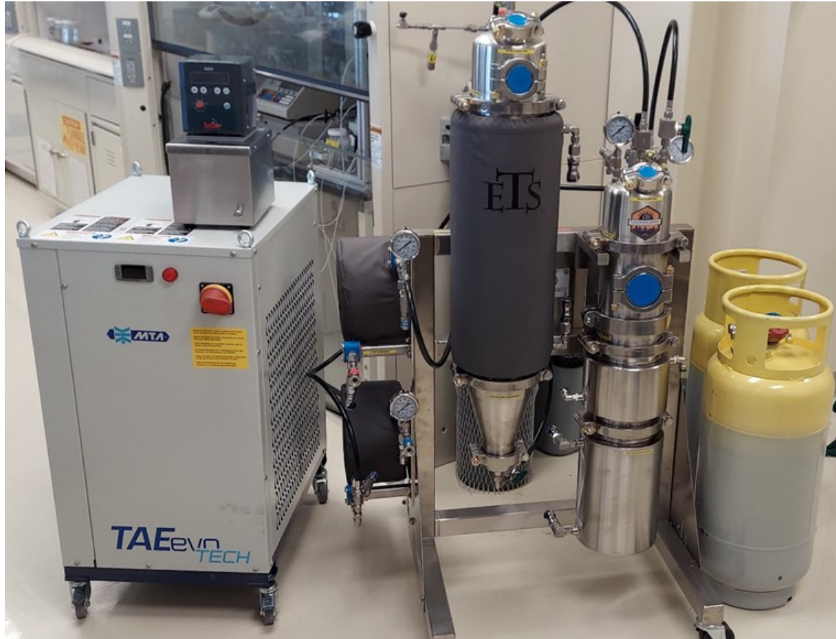
10L solvent extraction system
