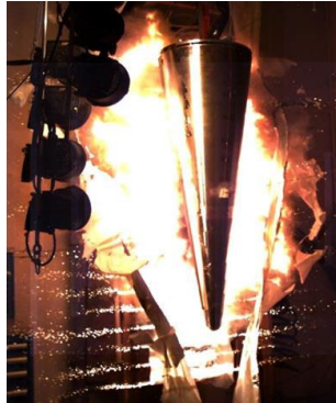
In-situ photograph of an LIHE Impulse Test at SNL on a surrogate warhead article. The high explosive was applied to the test article then initiated via high-energy light flashes.
