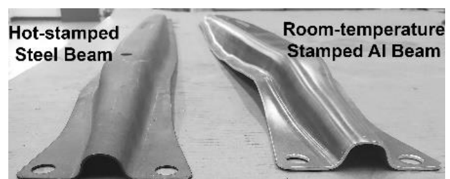
Figure 1. A side-by-side comparison of the production steel side-impact beam and the prototype high-strength Al beam.
