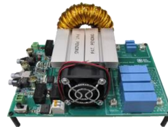
Figure 2. Picture of the hardware prototype with the High Flux core design, P3.
