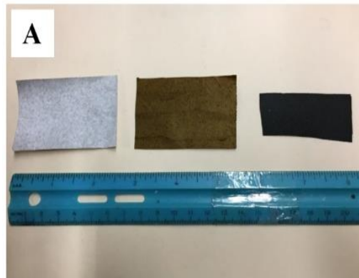
A. Simultaneous electrospinning and electro spraying, B. PAN/biochar precursor membrane, C. Stabilized membrane, D. Carbon nanofibrous felt.
