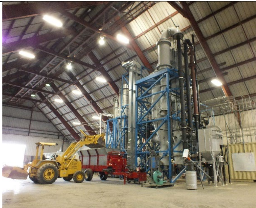
West Biofuels 5 TPD Dual Fluidized Bed Gasification System
