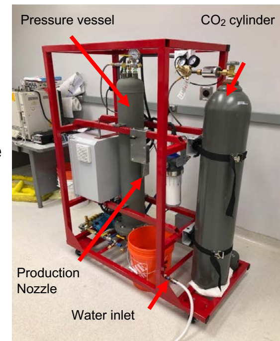
Lab-scale nanobubble generator
