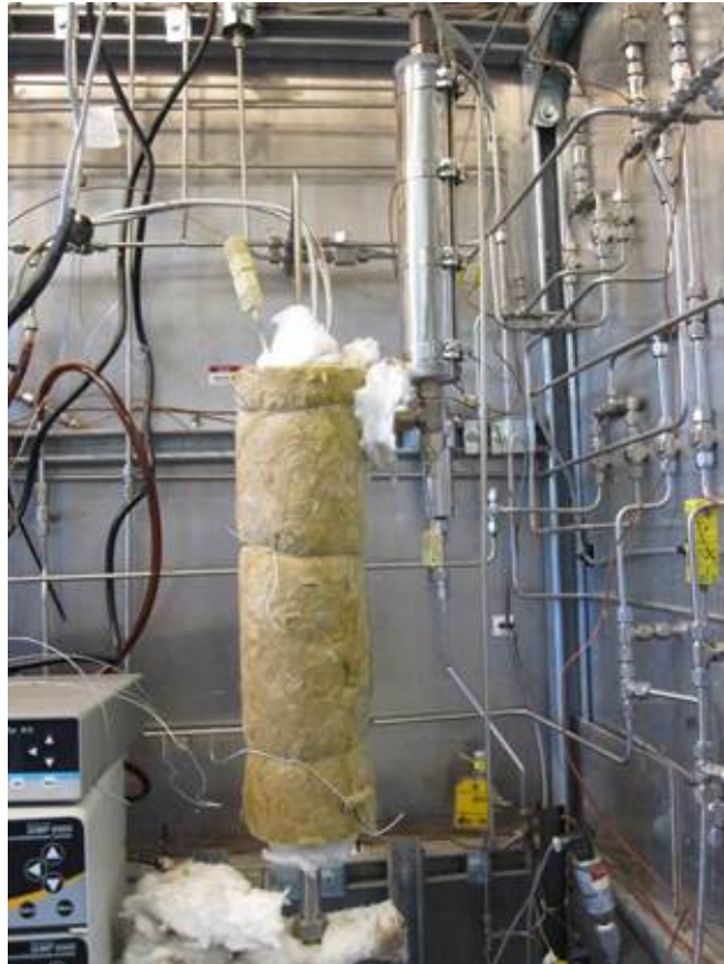
(3) Micro Scale CHG Systems 30ml Catalyst Bed 60ml/hr
