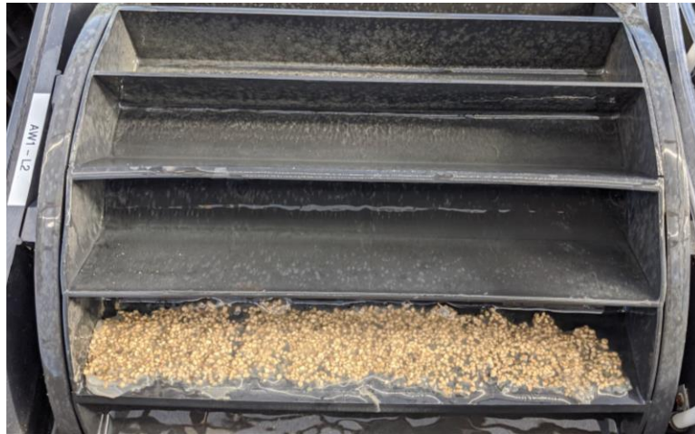
Before colonization: Algaewheel surface w/ and w/o adsorbents
