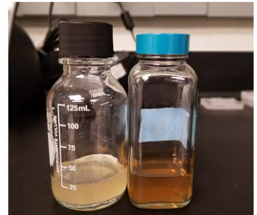
Extrusion produced liquor Left: Room temperature operation Right: 200°C operation
