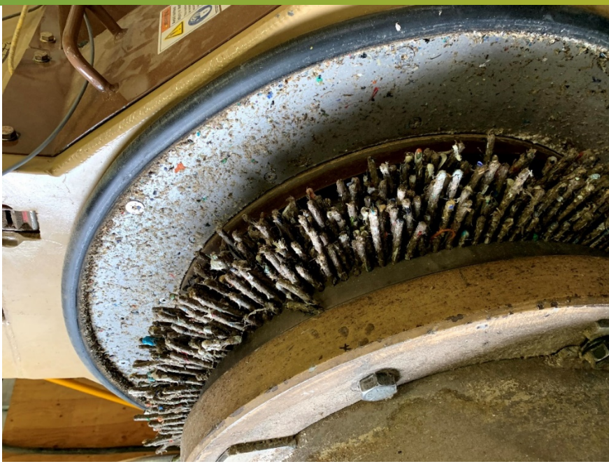
MSW pellets coming out of the pellet die.
