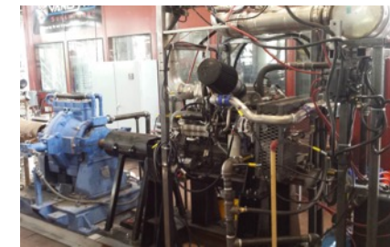
Cummins 6.7L QSB Tier 4 Final engine test cell (left). Pre and post catalyst PM10 emissions for ethanol-diesel fuel blends.
