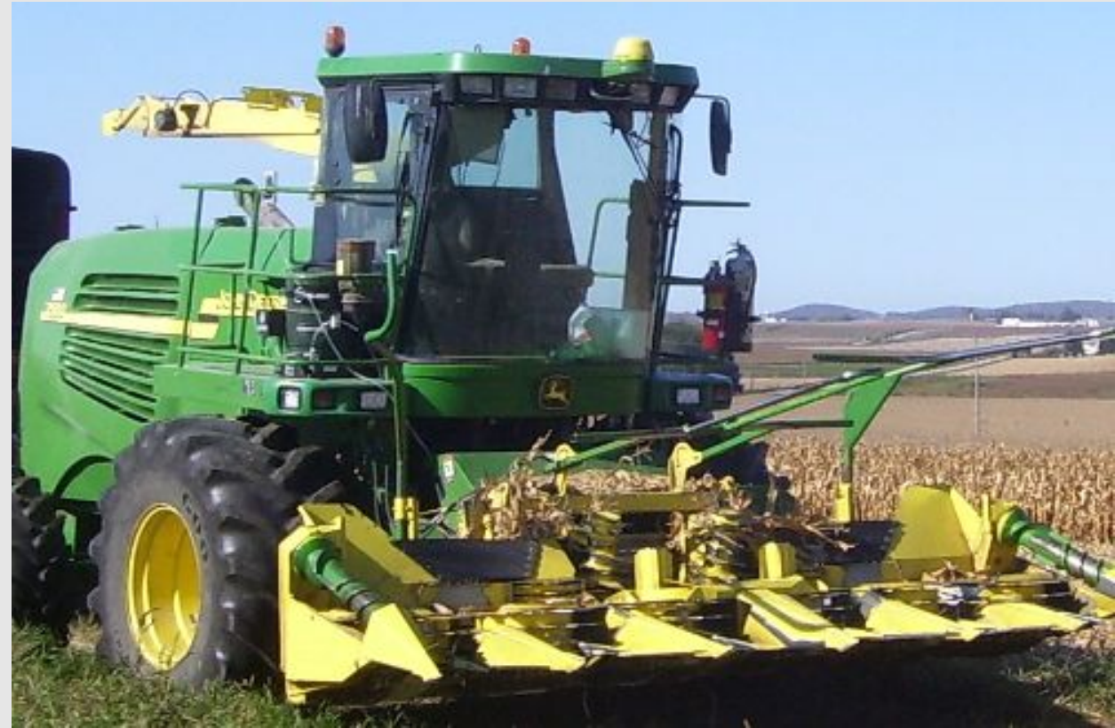
Forage harvester with ear-snapper (left) and whole-plant header (right)
