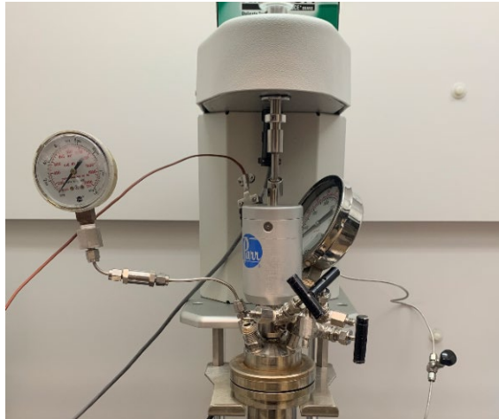
Bench-scale hydroprocessing to screen catalysts and process conditions
