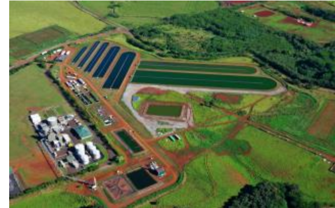
GAI's 33-acre algae facility in Kauai with CO 2 supplied from off-gas of adjacent power plant
