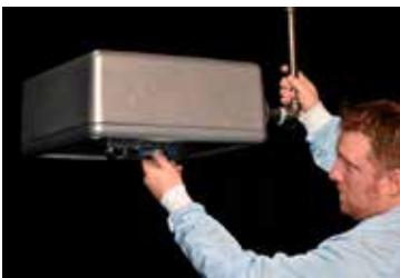
Figure 2. Luminaire mounted for photometry in a laboratory; note the orientation.
