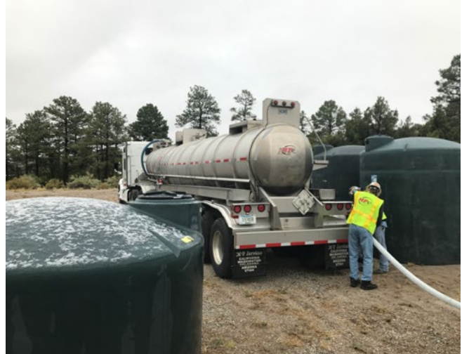
Workers prepare purged well water for shipment at the R-3 well pad in Pueblo Canyon.
