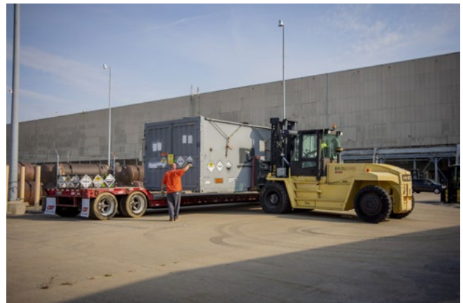
Cold traps are loaded for disposal, ranging in size and weighing as much as 15,200 pounds, about four times the weight of an automobile.
