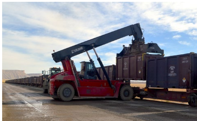
A reach-stacker lifts a container off a railcar at the Crescent Junction Site.
