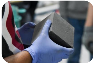
Example of grouted waste simulant
