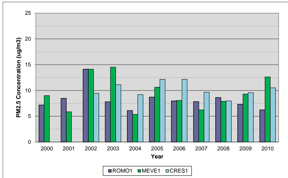
Figure 3-5. 98th Percentile 24-Hour PM 2.5 Concentration for the IMPROVE Monitoring Sites at Rocky Mountain National Park, Mesa Verde National Park, and Crescent Lake
