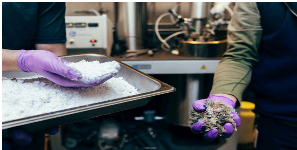
Figure 14. The IBM VolCat process selectively deconstructs PET in the presence of other waste
