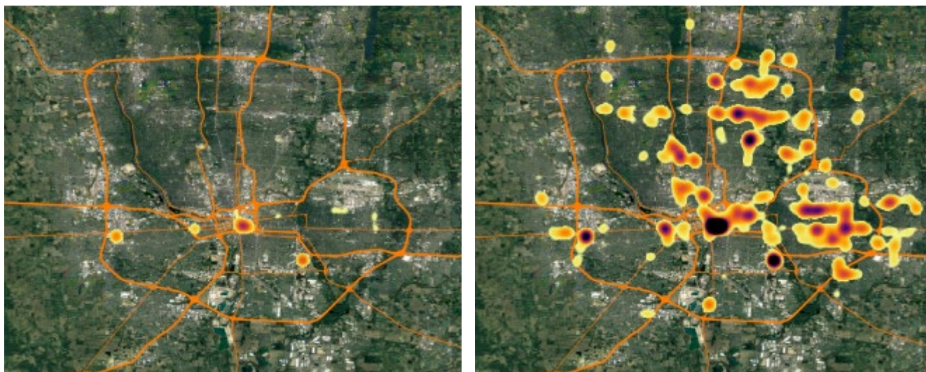
Figure ES-3. Heatmaps of simulated DCFC demand in Columbus, Ohio from electric taxi fleet with access to overnight charging (at left) and without (at right).
