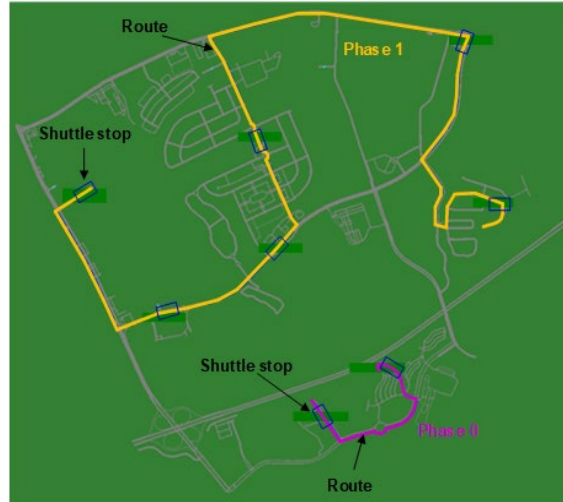
Figure 2-76. Greenville SUMO simulation network and fixed-route configuration.
