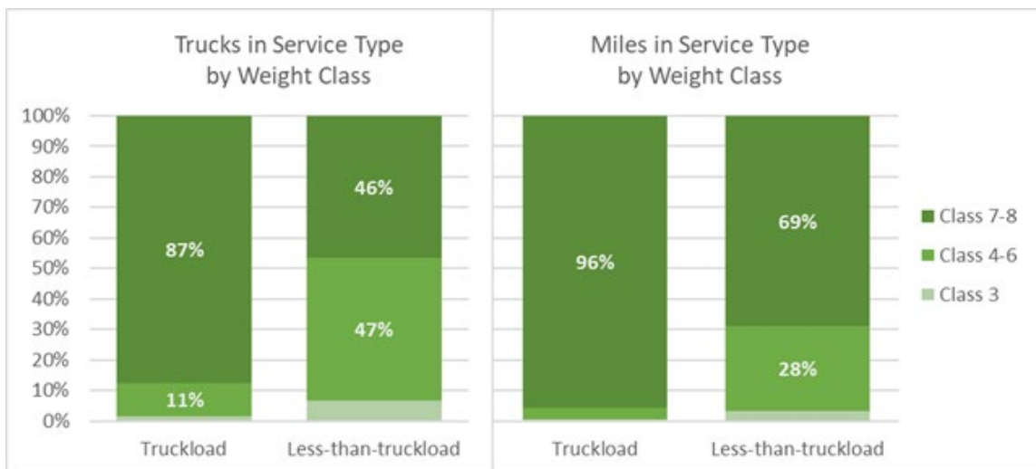
Figure 2-19. Distribution of trucks and miles by truck weight class for truckload and less-than-truckload service. Source: U.S. Department of Commerce, Bureau of the Census, 2002 Vehicle Inventory and Use Survey.
