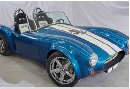
Using carbon fiber-enhanced polymers, the BAAM printer produced the frame and body of a full-scale Shelby Cobra in 2014; body panels feature a surface variation of 0.020 inches.
