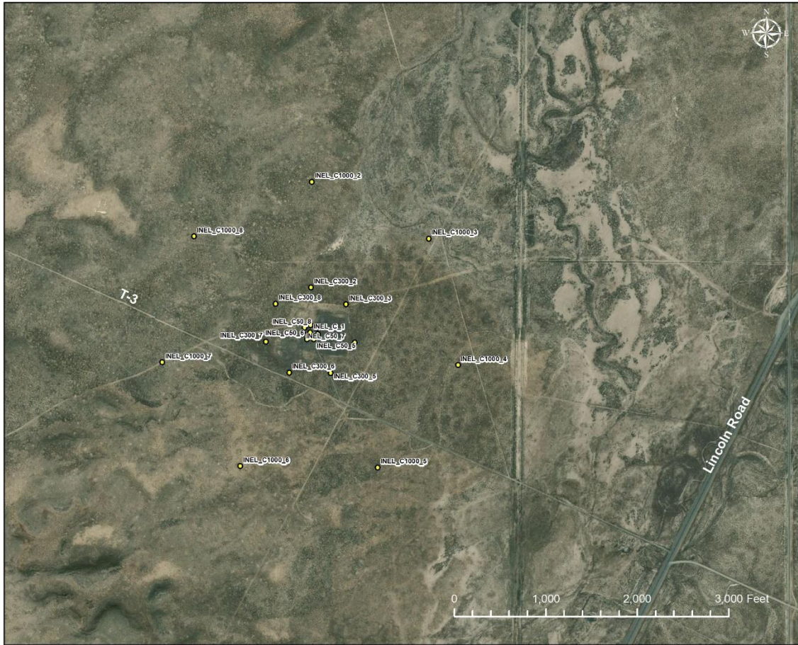
Figure R-13. Map of INEL-1 borehole site showing the proposed seismometer locations (labeled yellow dots) for the MAM surveys using three circular arrays, 165 ft (50-m), 985 ft (300-m), and 3,300 ft (1,000 m); MASW will be conducted within the smallest circular array.
