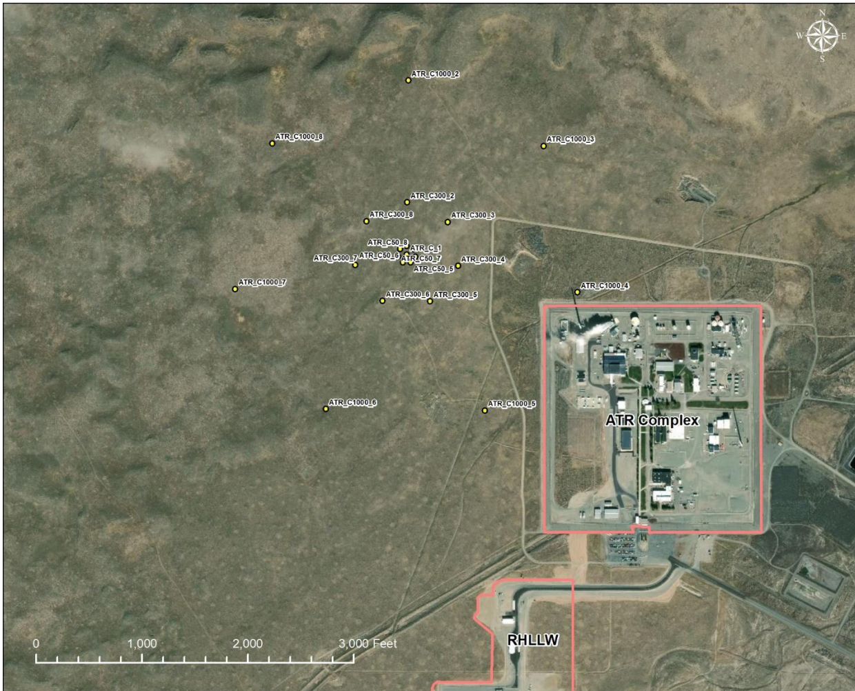
Figure R-9. Map of ATR showing the proposed seismometer locations (labeled yellow dots) for the MAM surveys using three circular arrays, 165 ft (50-m), 985 ft (300-m), and 3,300 ft (1,000 m); MASW will be conducted within the smallest circular array.
