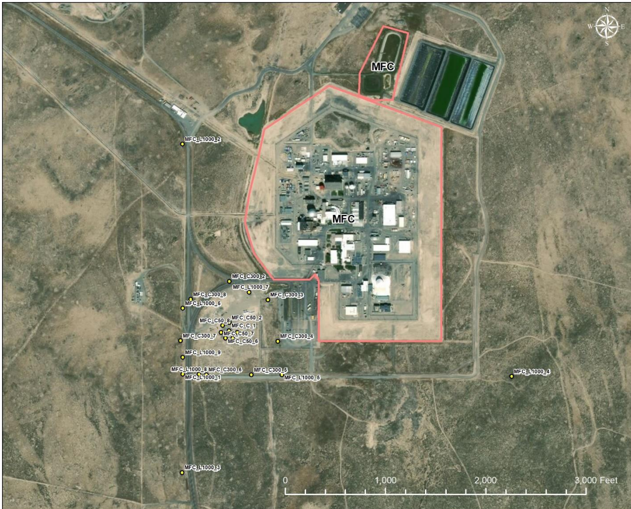
Figure R-10. Map of MFC showing the proposed seismometer locations (labeled yellow dots) for the MAM surveys using two circular arrays, 165 ft (50-m) and 985 ft (300-m); and an L-shaped array covering an aperture of ~3,300 ft (1,000 m); MASW will be conducted within the smallest circular array.
