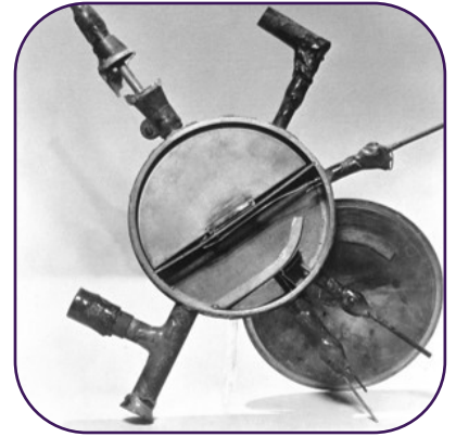
First working model of Ernest Lawrence's cyclotron Credit: Berkeley Lab Flickr (CC BY-NC-ND 2.0)
