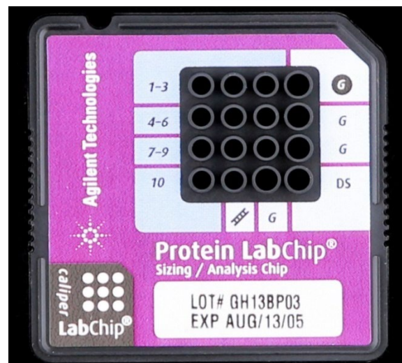
Caliper Life Sciences commercialized ORNL’s Lab on a Chip, which can analyze tiny samples of RNA, DNA, proteins, and other compounds—as small as a few millionths of a liter.
