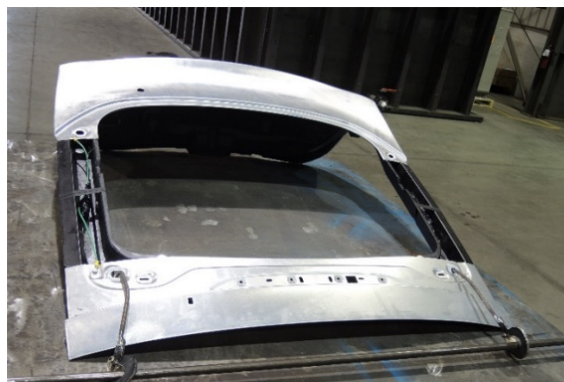
Figure 1. Prototype CFRP (black)/Al prototype liftgate.
