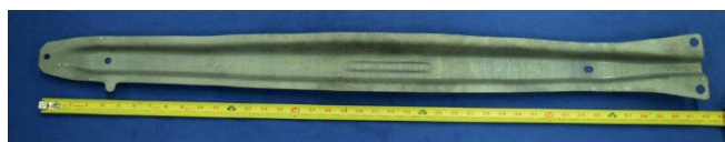
Figure 1. Top view of the steel side impact beam used as a reference to emulate high strength aluminum.
