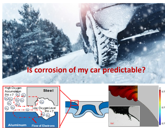
Figure 1. The mechanism of corrosion of dissimilar metals due to chemical reactions with the environment such as snow and salt. The reactions are illustrated on a SPR joint (bottom left) and mass loss due to corrosion (bottom right) and its prediction using the models developed by this project.
