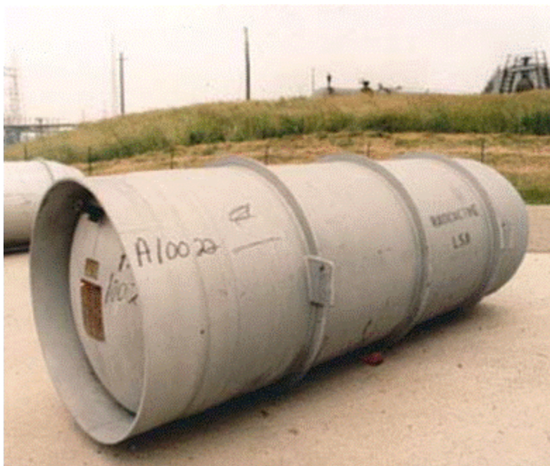
Figure 1-1 Typical Depleted Uranium Hexafluoride Storage Cylinder (Source: ANL 2001)
