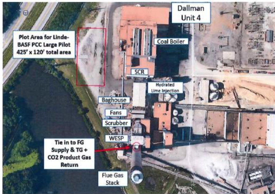
Figure 3 – Location of Pilot Plant on CWLP Facility
