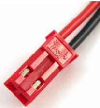
Figure 8. Competition-provided connector for manual shutdown interface
