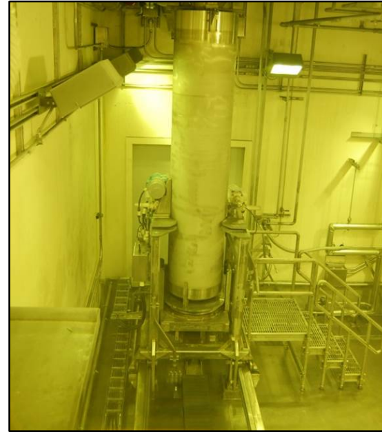
Can fill station at the Integrated Waste Treatment Unit
