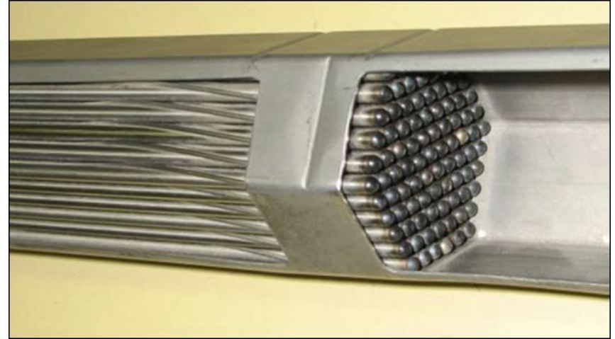
EBR-II driver fuel pins
