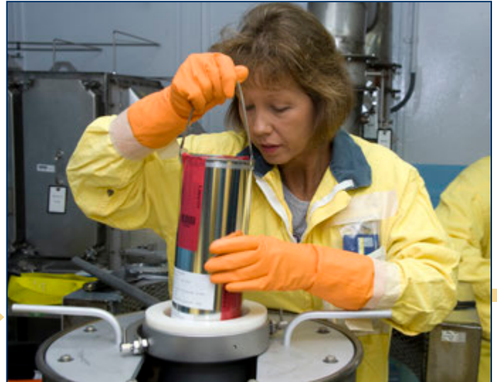
An employee packs a can into the ES-3100 shipping container for offsite shipment to Nuclear Fuel Services for down-blending. ES-3100s are routinely shipped via Office of Secure Transportation convoys.
