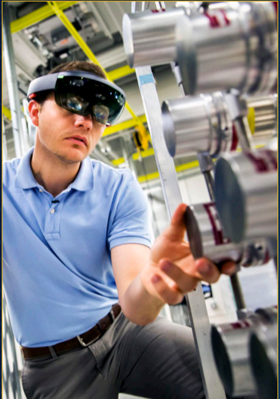
Michael Hamel, Nuclear Engineering and Radiological Science Ph.D. student, uses a headset with a radiation imaging array to demonstrate the use of augmented reality to find nuclear materials hidden in a room. Image credit: Joseph Xu, Michigan Engineering
