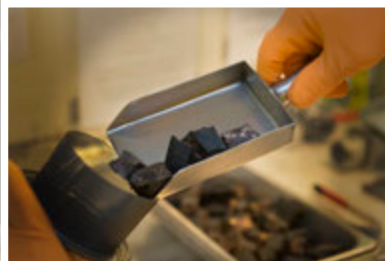
Broken uranium metal from a hollow log casting is being packed into an offsite shipping can. The can is lined with a metal screen to protect it from potential sharp edges of the material. This material was produced using existing supplies of highly enriched uranium. The can of metal will be packaged into an ES-3100 shipping container and shipped to Nuclear Fuel Services for down-blending.
