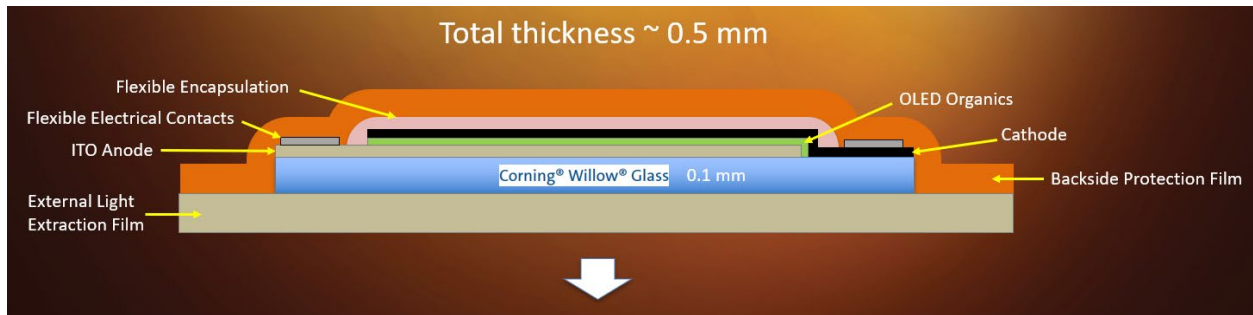
Figure 4.24 Encapsulation structures for conformable OLED panels. [62] Figure shows a conformable OLED structure that uses ultra-thin glass and a backside protective film that enables both conformability and protection from the ingress of water into the OLED device structure.
