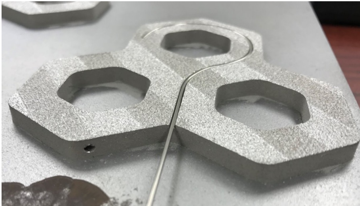
316L sheathed sensor in AM 316L build
