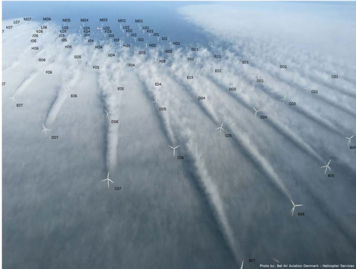
Figure 2. Photograph of Horns Rev. 2 wind plant from January 25, 2016, showing individual wind turbine wakes delineated in the fog with clearing in the overall plant wake downwind of the wind plant. Photo by Bel Air Aviation Denmark–Helicopter Services.
