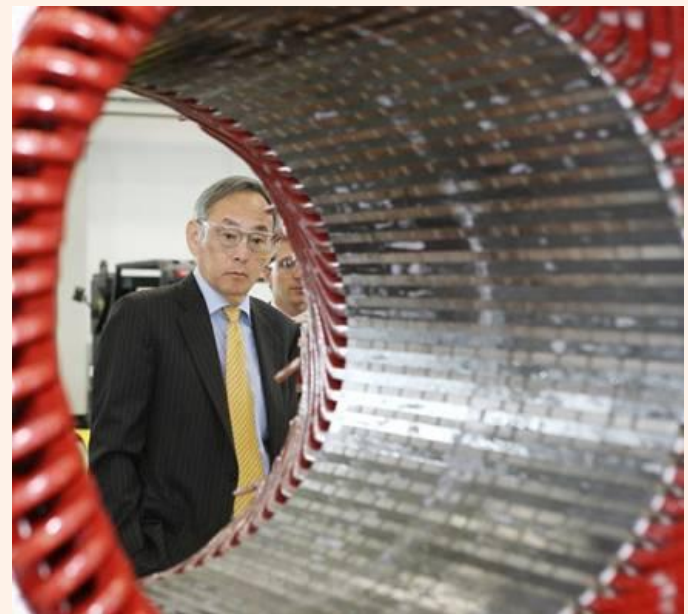
Secretary Chu visiting Ingeteam Inc.'s Milwaukee, Wisconsin facility. In this photo he is looking at the stator of a 2MW Wind Turbine Generator.
