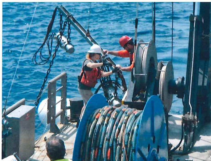
Figure 2: USGS scientists retrieve a pair of airguns and the gun hanger during the 2018 MATRIX cruise. The seismic streamer is coiled on the blue winch in the foreground. (Courtesy of USGS).
