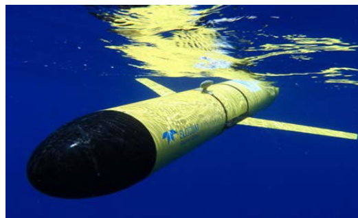
Figure 3.4. Teledyne Webb Research's Slocum glider. Image courtesy of WHOI
