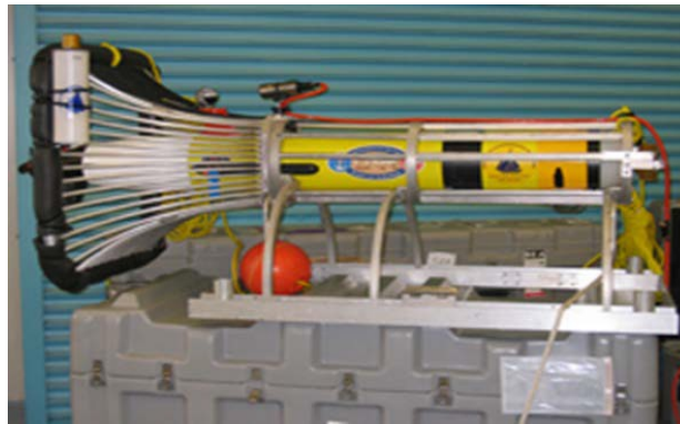
Figure 3.2. Underwater Remus docking station. Photo courtesy of Woods Hole Oceanographic Institution (WHOI)
