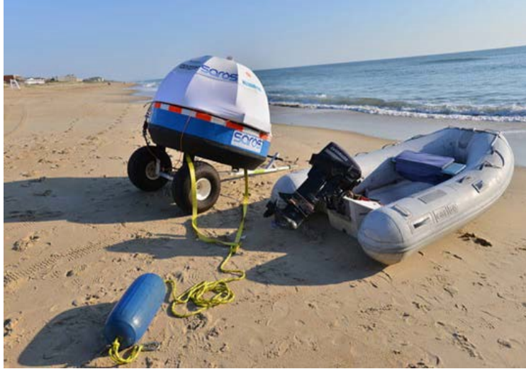
Figure 7.4. SAROS wave-powered desalination demonstration unit
