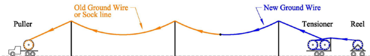
Figure 2-4. Typical Stringing Operation
